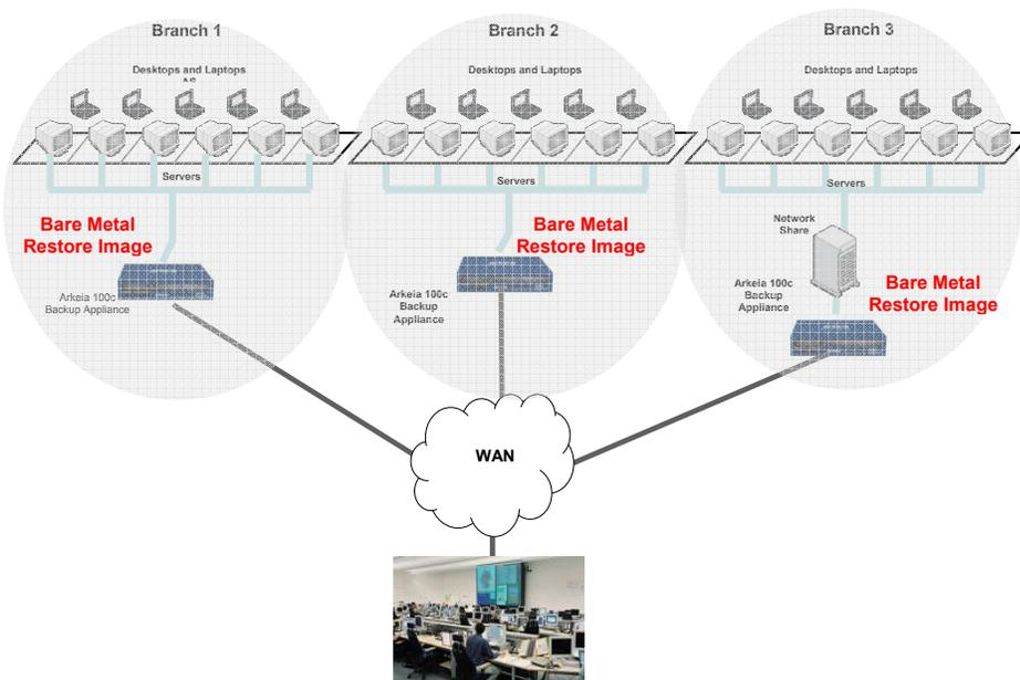
In each branch office, a disk and tape EdgeFort is installed. Mission critical workstations are imaged and stored locally for rapid recovery. The image may be stored on an EdgeFort disk or tape. Supporting a bare-metal restore with an EdgeFort added allows for even greater remote office data protection, reduced risk and shorter time to recovery.
